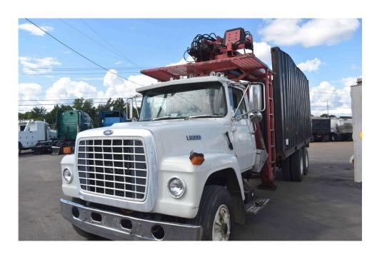
1985 FORD, L9000, Heavy Duty Trucks - Grapple Trucks, CATERPILLAR 3406B, Manual, good truck, runs great, differential lock, IMT 16000S2 boom and grapple, 40 yard box, 400 Horse Power, Air Ride Suspension, Wheels, Wheel Base, , Axle, Ratio, , VIN 1FDYU90X5FVA51638
