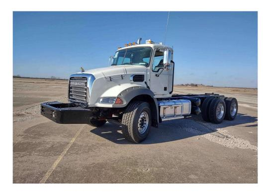
2024 MACK, GRANITE 64BR, Heavy Duty Trucks - Cab & Chassis Trucks, MACK MP8, AMT, MP8 455HP, mDrive HD 13 Spd, Fa: 20K, RA: 46K on mRide, Disc Brakes, 27" Front Frame Extension.
