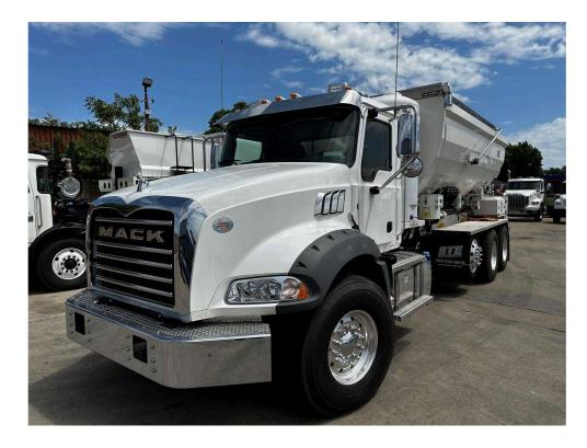
2023 MACK, GRANITE 64BR, Heavy Duty Trucks - Mixer Trucks / Asphalt Trucks / Concrete Trucks, MACK MP7, Automatic, 2023 Bay Lynx "TITAN" Volumetric Mobile Concrete Mixer. Made with Hardox Steel. INCLUDES: Bay Lynx BatchPRO 3.0 computer-controlled info system, 350 cu. ft. aggregate bin with two vibrators, extended conveyor, hydraulic metering gates, 106.5 cu. ft. cement bin, 500 Gallon poly water tank, HD Mix auger, Admix system, Fiber, Color and many more
